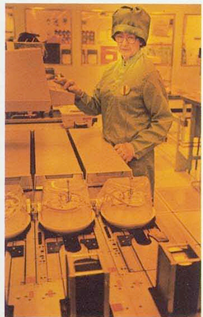
Patterns are produced on the wafer which define the outline of the chip as well as the components on it.
