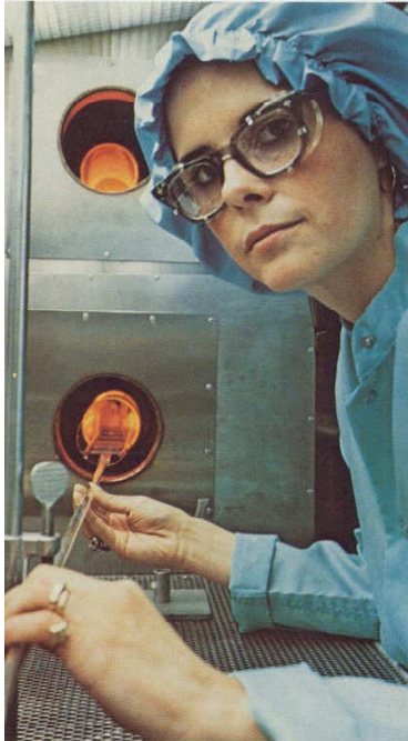
Impurities are diffused into the wafers in ovens set at about 1000 degrees Centigrade.
